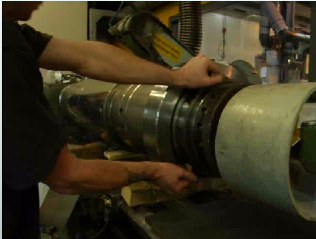
Impeller pitch control axle Spanish hydro-electric power plant.
