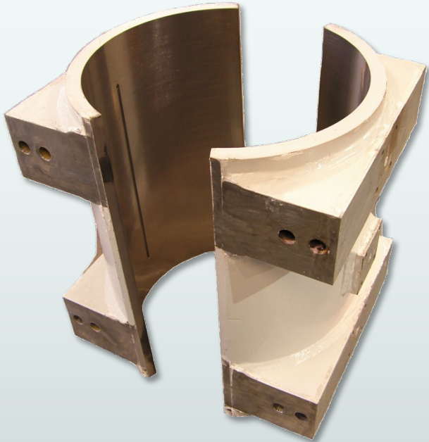
Disk spring guidance (Ketelbrug). Lunac 2+ coated for reasons of anti-fretting/anti-galling and stable coefficient of friction
